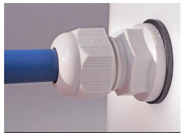
Putting cables into an entry hole without a gland not only puts stress on the cable's termination, i.e. terminal block or cable lug, but also allows solid objects and liquids into the enclosure that can cause issues over time or prevent proper IP ratings from being achieved.
